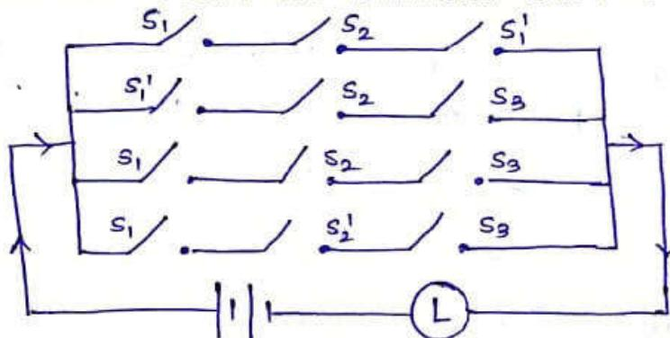
Q4 Represent the following switching circuit in symbolic form & construct its switching table. Write your conclusion from switching table.
